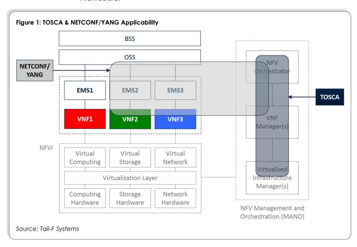
In a service fulfillment scenario, where new instances of VNFs need to be created, NFV MANO will be responsible for unpacking TOSCA templates to understand what resources the VNFs will need. Working together, the different orchestration layers of the NFV MANO stack will use the VNFs' deployment templates to create the required
